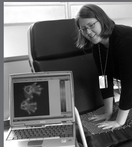
Laurie DeLaney, an occupational therapist and assistive technology practitioner with the CC Rehabilitation Medicine Department, demonstrates the department's pressure mapping system. It evaluates pressure distribution in wheelchairs and beds and shows patients and nurses areas at risk for pressure ulceration.
